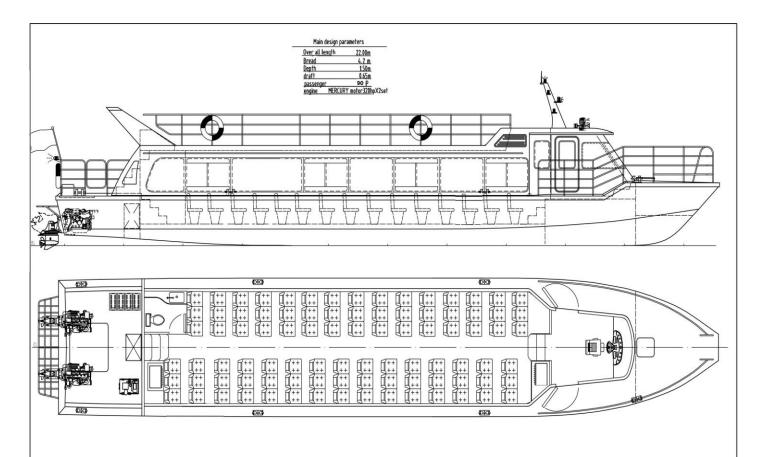
$22 \mathrm{m}$  layout, 90 passengers, outboard or stern drive inboard engines
